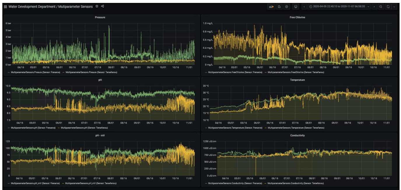
Figure 30: Measurement time-series from a multi-parameter sensor installed in the WDD network
