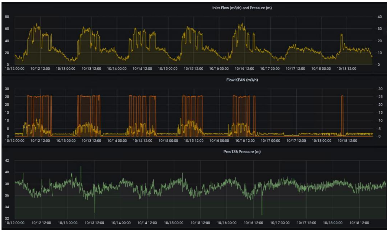
Figure 9: Measured inlet flow, inlet pressure and KEAN factory consumption of DMA 136 received from installed sensors for the period 12-18/10/2020.
