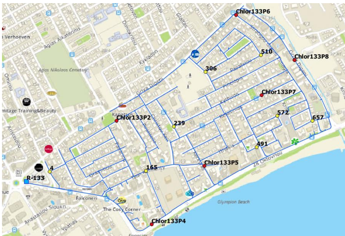
Figure 26: GIS map showing the location of the chlorine sensors (red) installed in DMA 133 and the locations where field measurements were taken (yellow)
