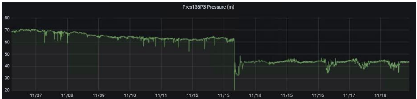
Figure 43: Measured pressure of Pres136P3 sensor of DMA 136 for the period 7-18/11/2020.
