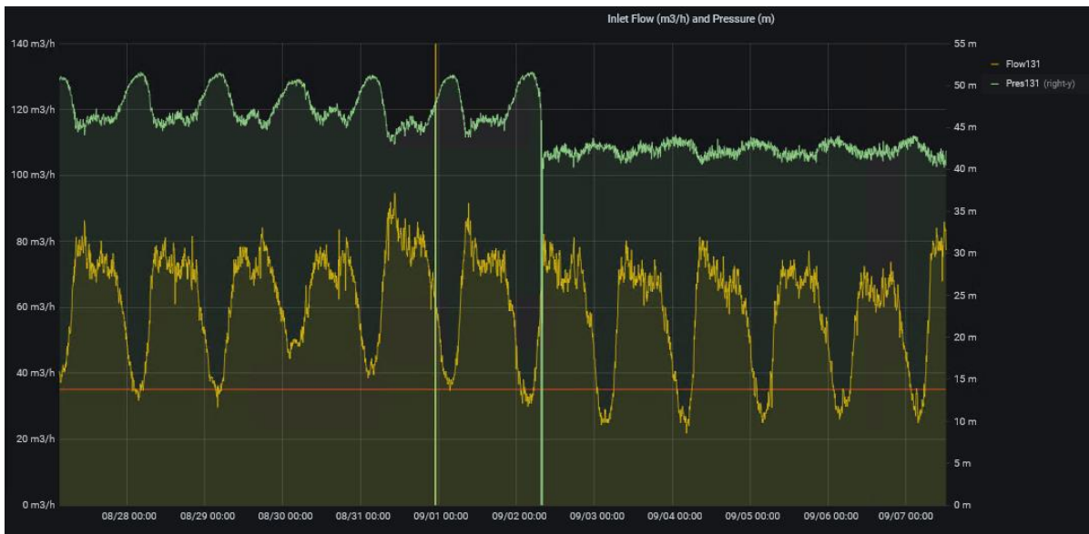
Figure 57 - Reduction of minimum night flow in DMA 131 when applying the pressure control algorithm
