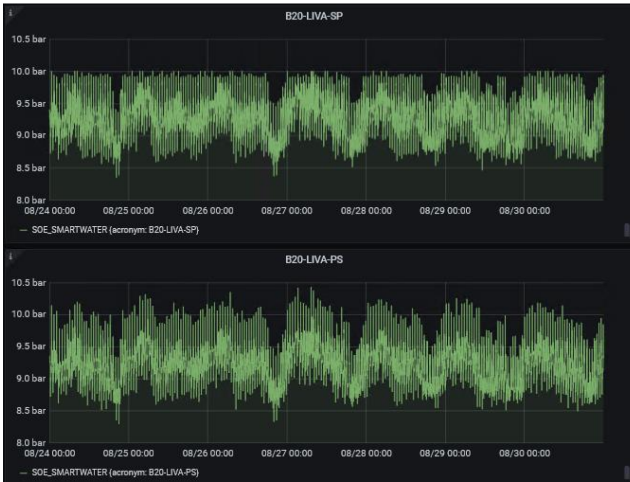
Figure 19: Measured upstream and downstream pressure at the Leivadia Pump Station for the period 24-31/08/2020. Pump station was not operational during that time according to the general operational scenario of the entire network.
