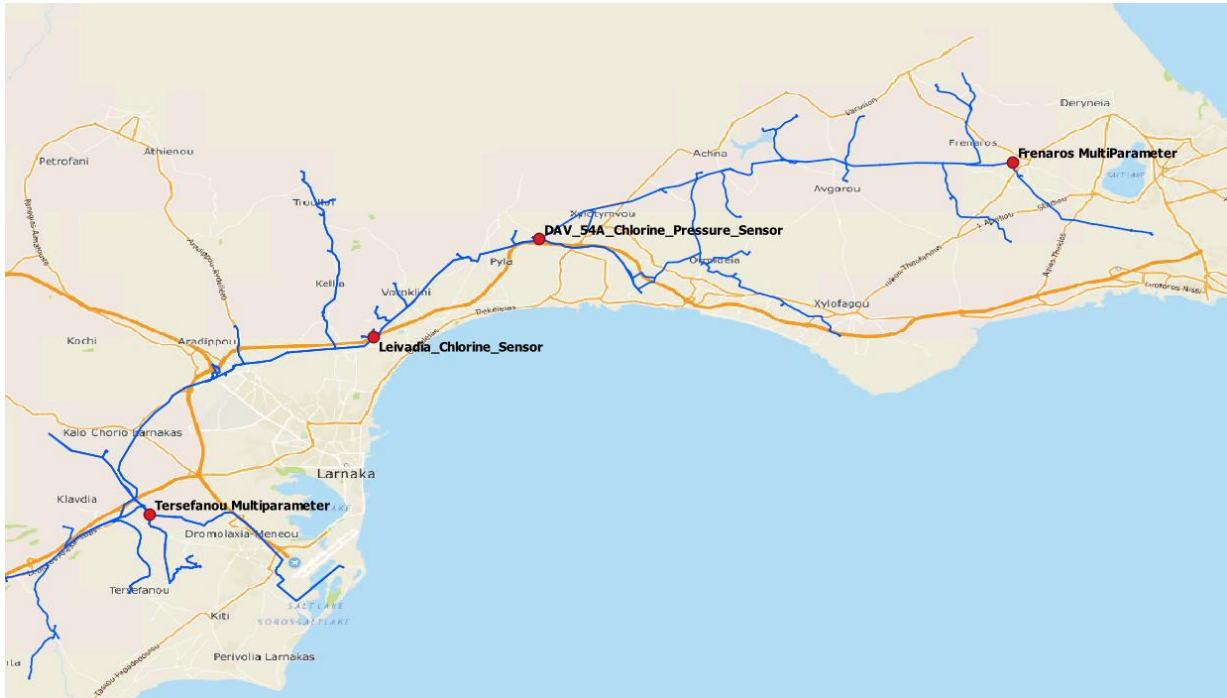
Figure 29: GIS map of the locations of chlorine and multi-parameter sensors in WDD network.
