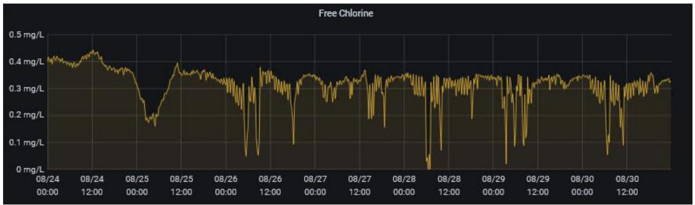
Figure 31: Chlorine concentration measurements from the “Tersefanou” multiparameter sensor for the period 24/08/2020 - 31/08/2020.
